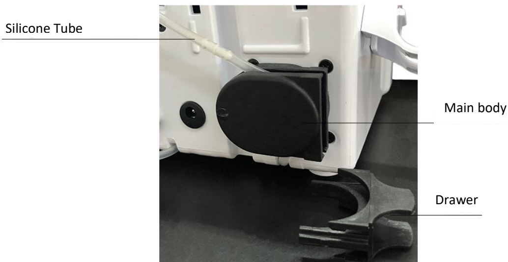
Figure 5: Items that make up the peristaltic pump.
