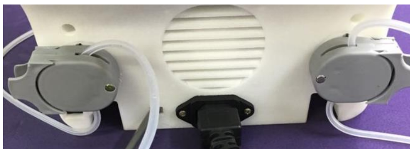
Figure 3: Peristaltic pump assembled to the DentSurg Pro equipment
