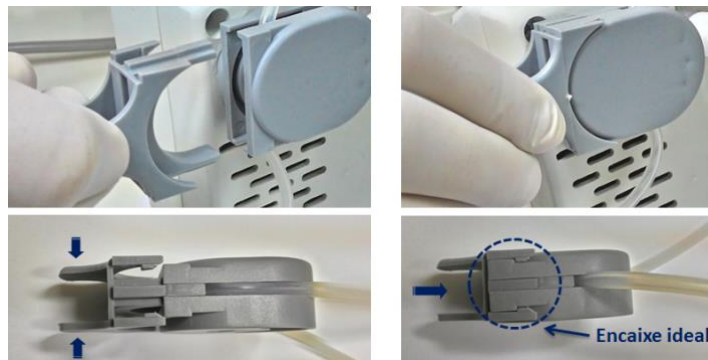
Figure 5: Reposition the silicone tube, press the tabs of the locking part and push it towards the pump head, until it reaches the ideal fit.
