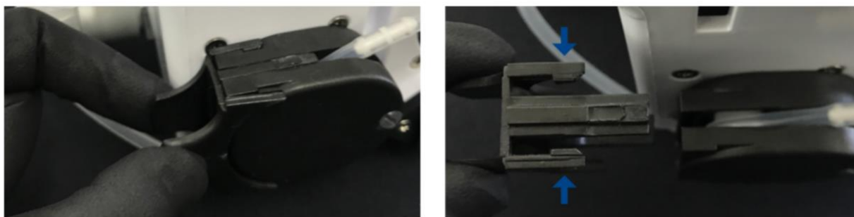
Figure 7: Press the drawer fins (one against the other) and pull it out, allowing free access to the silicone tube.
