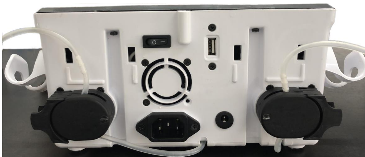
Figure 6: Peristaltic pumps assembled on CLINICAL PLUS equipment.
