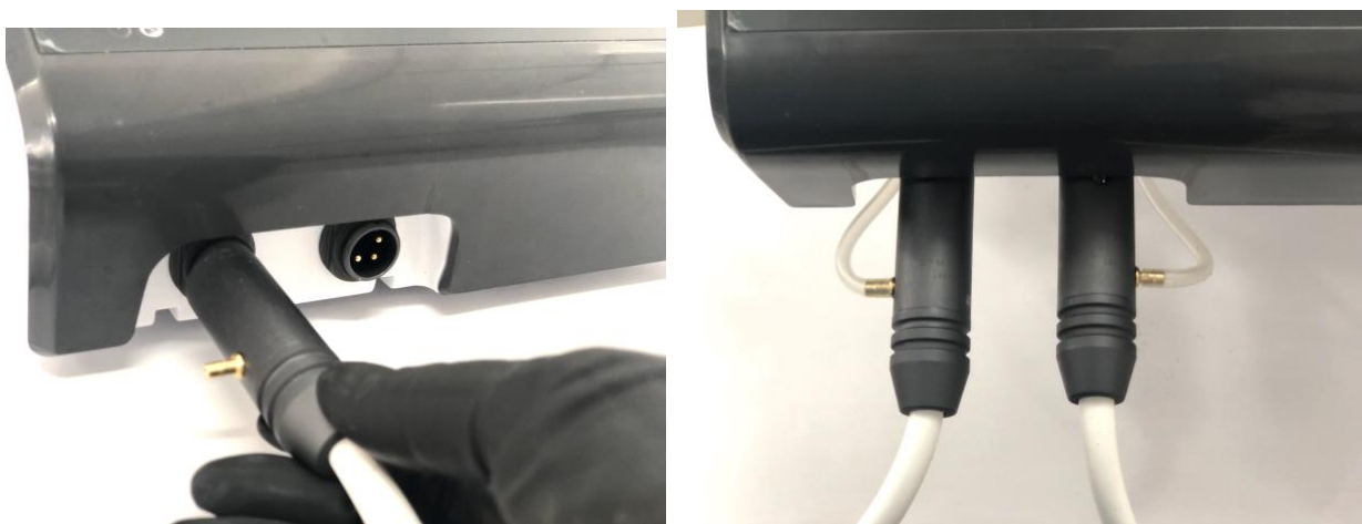
Figure 13. Connecting the handpiece to CLINICAL PLUS ultrasound equipment
