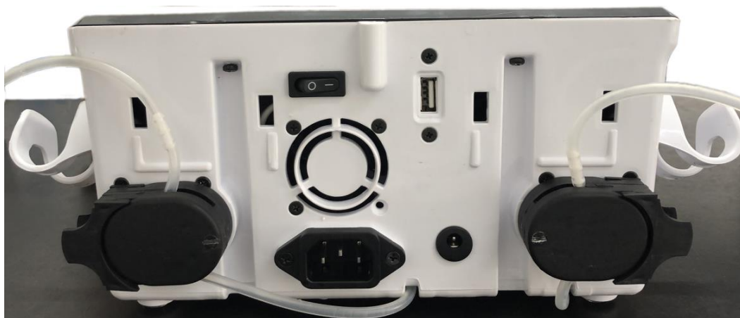
Figure 14. Back of CLINICAL PLUS ultrasound equipment, place of the on-off power button.
